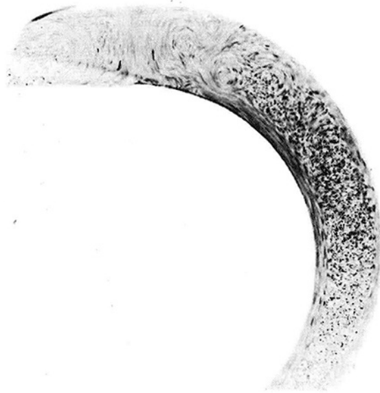
Fig. 2 Multiple vortex flow pattern for 350 fluid, D = 1.40 , e/L = -0.375
